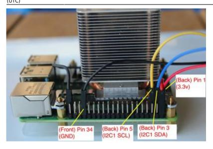
RTC (Real Time Clock): Attach to Raspberry Pi
