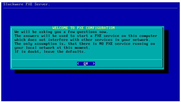
A working DHCP server is required for PXE boot. So, if your network does not provide one, pxesetup will start its own built-in DHCP server and it will show you two additional dialogs in order to collect the required information:
