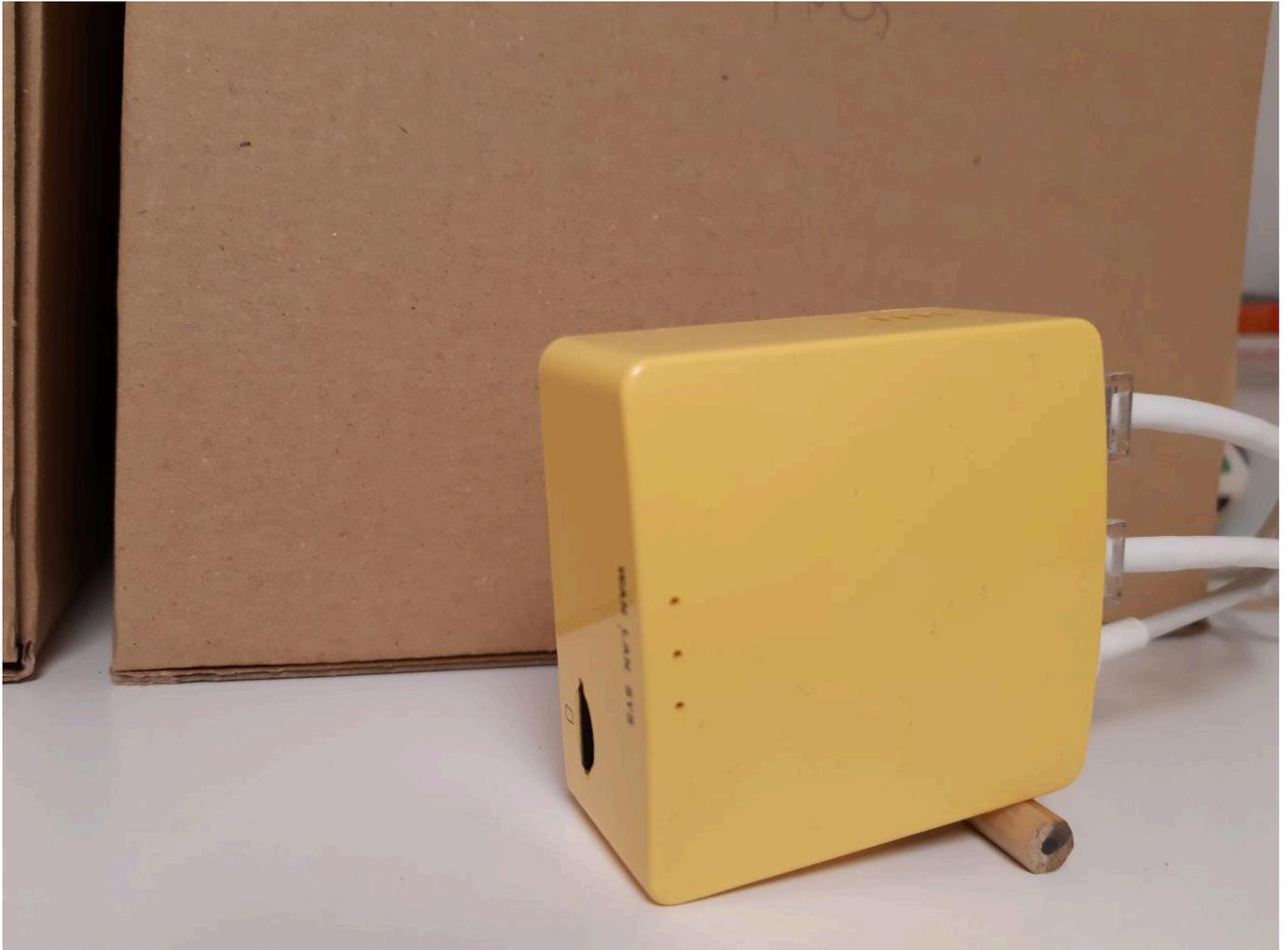
The original case has 2 issues: cappy internal antenna and tendency to overheat ... so I 3d-printed my own [case](#).
