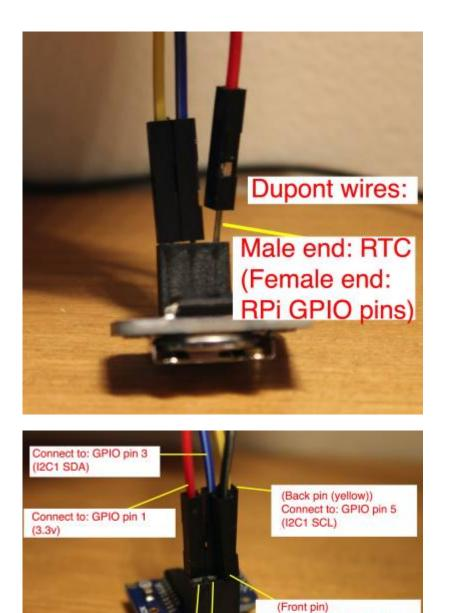
Empty front pins Connect to: GPIO pin 34
