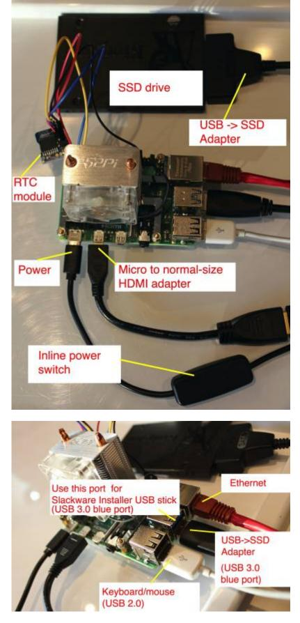
The basic hardware setup is complete.
