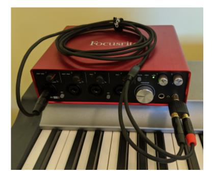
After all connections are made, jack\_iodelay will report the full loop latency, in milliseconds, frames (samples), how much of the latency is due to hardware (it does this by subtracting the known latency from the total measured), and also recommends values to set for input and output ports.
