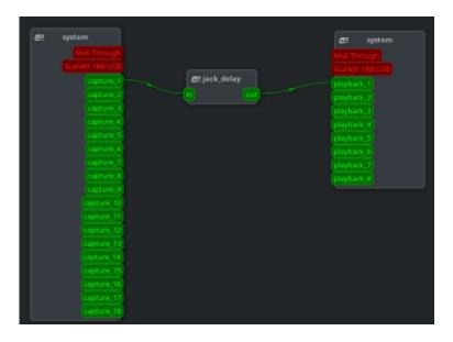
The last step is to connect the physical output back to the physical input that jack\_iodelay is using. Also don't use an output with speakers, the program uses a series of tones to measure latency and you probably don't want to hear them.
